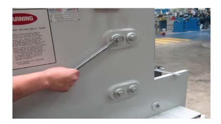
Use front and rear jacking bolts to set the required blade gap to suit material being cut.
